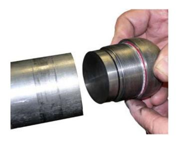
6. When properly installed, the rotor may be heard to hit the housing when the vibrator is struck smartly against the palm of the hand.
