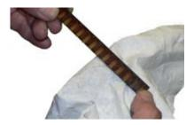
7. If a new vane does not fit closely in the rotor groove, replace the rotor. The rotor should be round, with all surfaces smooth and ungrooved.
