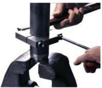
4. Once the threads start to unscrew, clamp the vibrator horizontally in the vise and remove the nose cap. The wear plate should come out with the nose cap. Keep them together.
