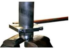
3. While still hot, use the tube wrench (or pipe wrench) to break the main body loose from the nose.
