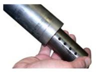
6. Examine the vane for grooving and signs of wear. If there is any noticeable wear on the vane or it does not fit in the groove of the rotor closely - replace the vane.
