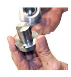
5. Carefully install the nose cap/wear plate assembly back into the vibrator housing. Screw it in about halfway. Apply thread locking adhesive to the threads (3-4 drops) and continue to tighten the nose cap until it is secure.
