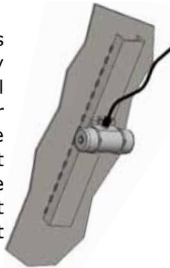
Single Phase models: **Mount vibrator with the power cord facing upwards.**
