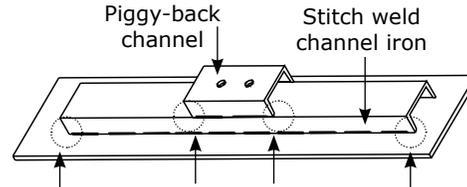
*Do not weld the ends of the channel iron. This allows the vibrational force to "escape". Solid welded ends trap the force, which can cause stress cracks.*
