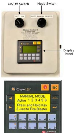
Mode Switch: The Mode switch is used to select the desired operational mode - Automatic, Manual, or Remote. Mode of operation can be changed at any time regardless of whether the power is on or off.
