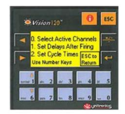
**Channel Activation:** Regardless of the Mode of operation (Manual, Automatic, or Remote), a timer channel must be ACTIVATED before it will fire. From the Configuration Menu, press the "0" Key to open the Select Active Channels screen. A screen similar to the one below will appear.
