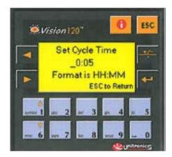
In the example above there is a delay of five minutes after each cycle ends before the next one is activated. The missing digit above is actually flashing to signify it can be changed with the keypad. Enter the desired setting using the numbered keys on the keypad. If you make a mistake you can use the LEFT ARROW key to go back a place. After entering the setting, press the ENTER key to record the setting. Press the ESC key to return to the original MODE screen.
